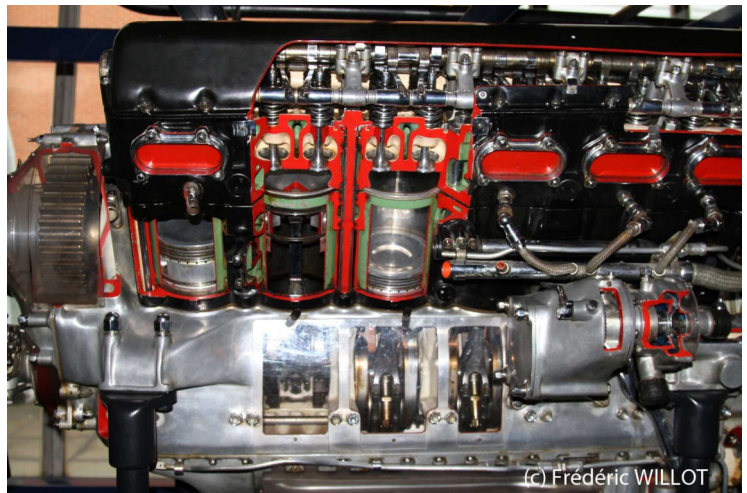
V shape d18 cylinder piston engine.
